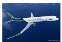
The first concept, a turbofan aircraft with a range of around 2,000 nautical miles (3,700 km).
